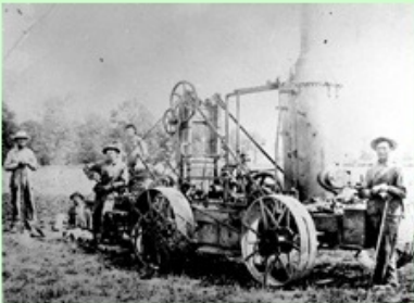
Drainage of farmland has always been a problem in the Great Black Swamp. The Buckeye Traction Ditcher (pictured here near Hamler, Ohio in 1905) was a successful attempt to help farmers keep more land under cultivation with less work. CAC General Photograph Collection. For more recent related material, researchers may wish to refer to the William F. Wittenmeyer/Garwood Buckeye Traction Ditcher Collection ( MS 380 )
