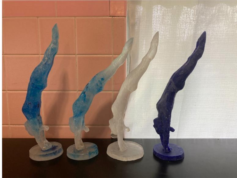
**Figure 1:** From Left to Right – Cu powder, Cu foil, no color added, and cobalt frit
