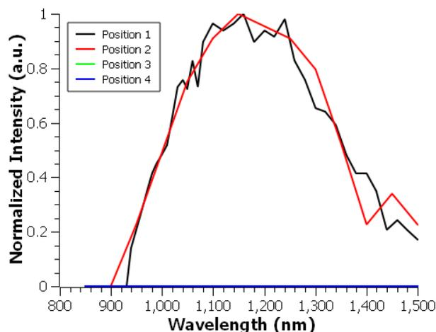
**Figure 5:** Normalized PL data showing the signal of BSA-QDs on a glutaraldehyde substrate. (Position 1) was located on the border of the BSA-QDs and a section of glutaraldehyde. (Position 2) was located amidst the BSA-QDs. (Position 3) was amidst the glutaraldehyde. And (Position 4) was on the wafer only.
