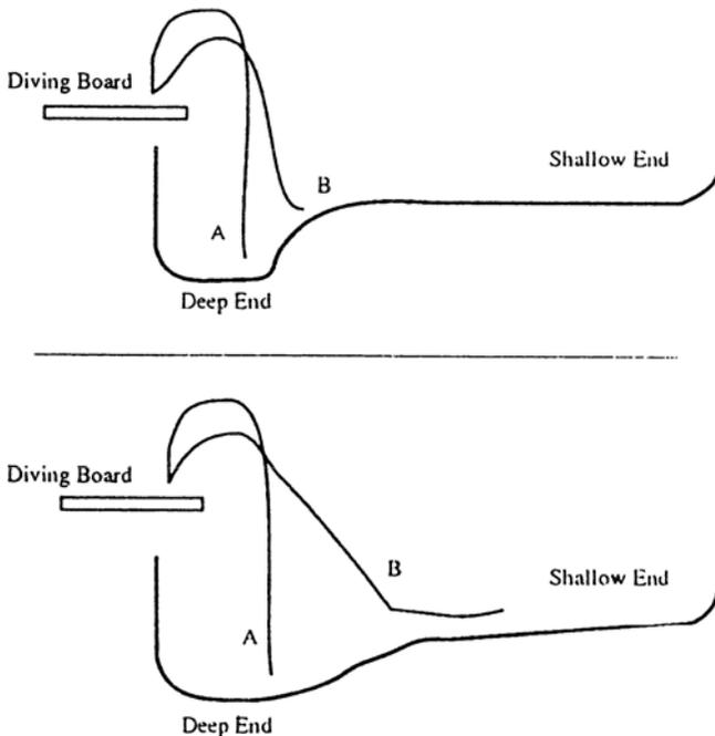
**Figure 2** — Different deep end configurations (from Laughery et al., 1992). Reprinted with permission.
