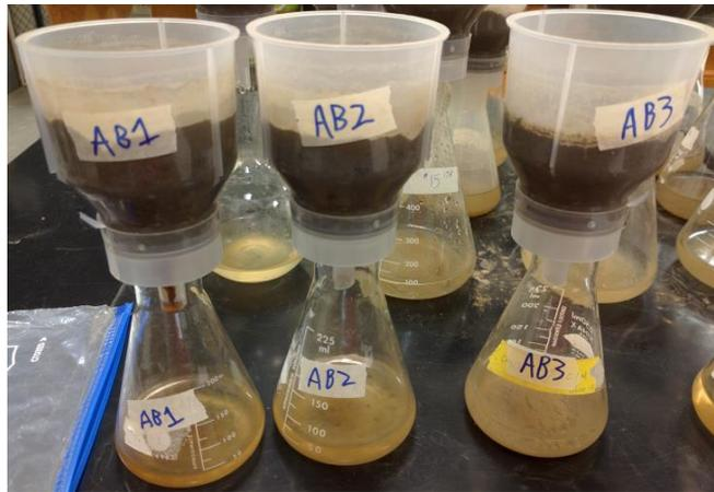
**Figure 5:** The above figure shows the apparatus for the rain simulation procedure.
