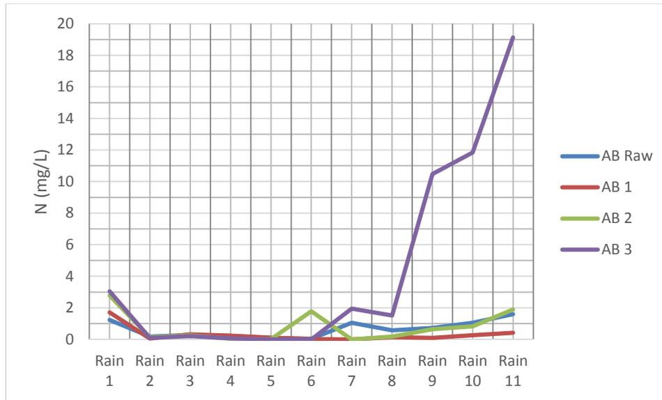
**Figure 8:** This figure shows the release rate of nitrate + nitrite under ambient light.
