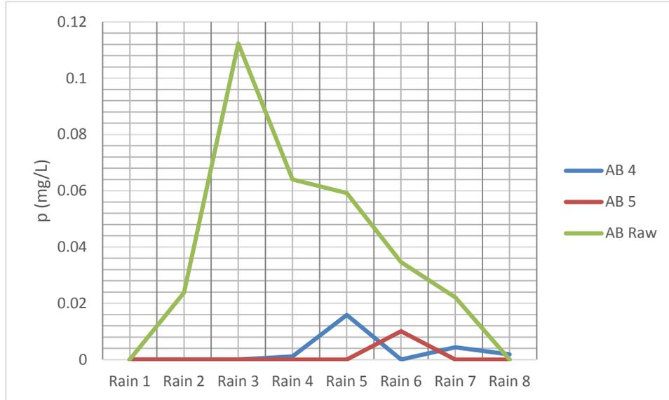
**Figure 9:** This figure shows the release rate of ortho-phosphate under ultraviolet light.
