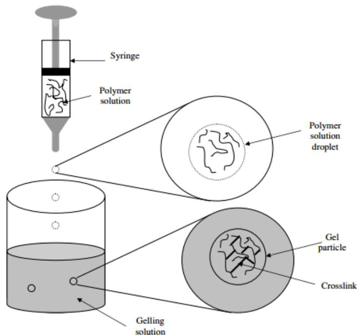
**Figure 2:** The process of extrusion to form gel particles (Burey 2008)
