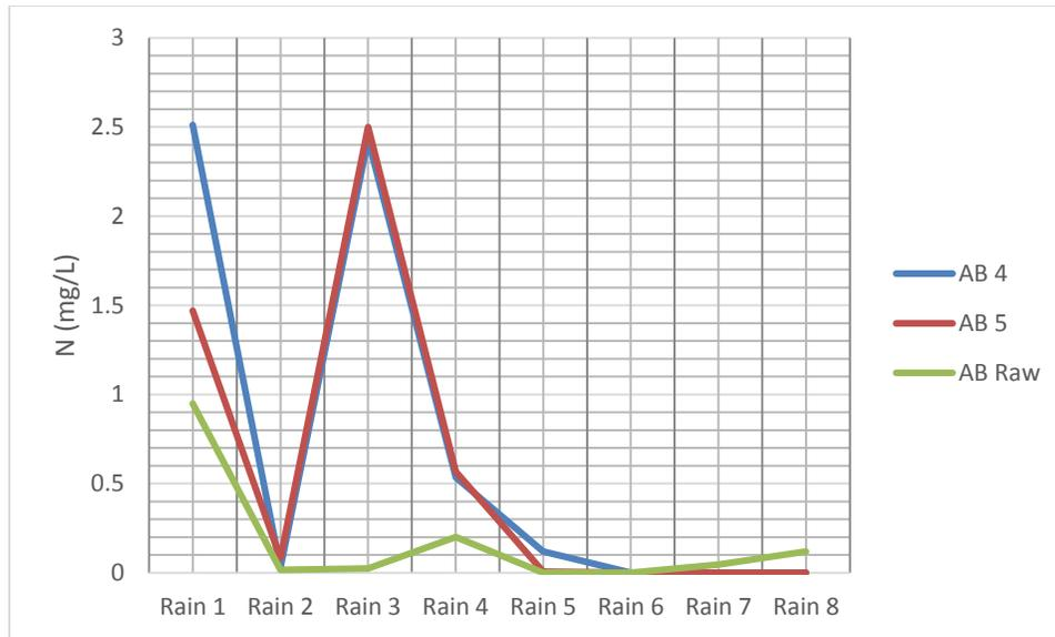
**Figure 11:** This figure shows the release rate of nitrate + nitrite under ultraviolet light.
