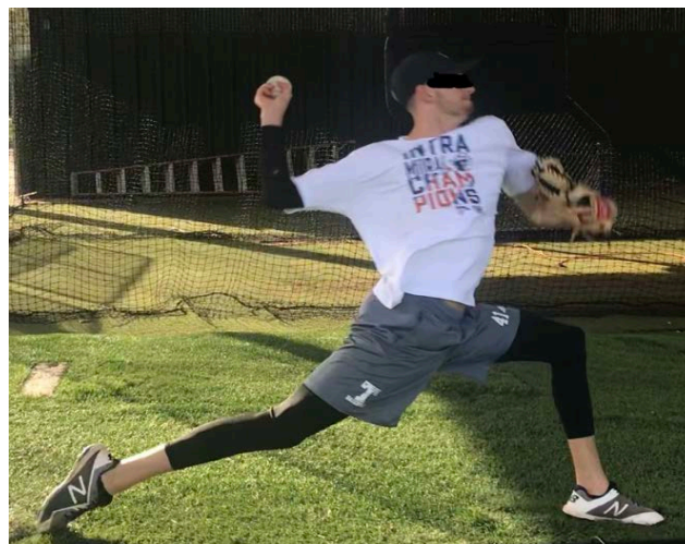
Figure 1. Subject throwing from 10-inch mound with 3D motion sensor sleeve on his throwing arm.
