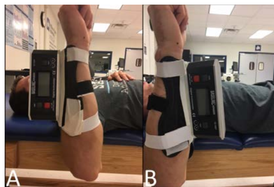
Figure 1. Purpose-built sleeve to secure digital inclinometer for glenohumeral external (A) and internal (B) rotation.
