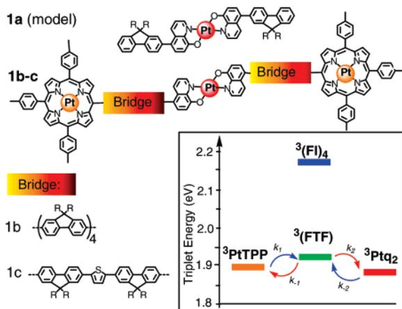
**Figure 1.** Structures of **1a–c**. Inset: Schematic representation of the triplet energy alignment in **1b** and **1c**.<sup>11</sup>
