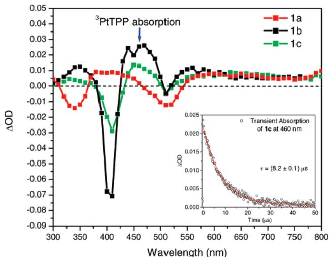
**Figure 3.** Transient absorption spectra of **1a–c** 200 ns after excitation at 510 nm. Inset: Decay trace of **1c** at 460 nm (<sup>3</sup>PtTPP absorption).
