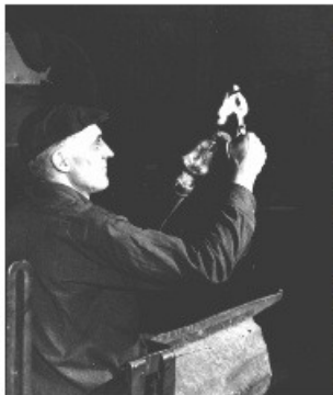
▶ A workman attaches molten glass to form the foot of a piece of stemware. Tiffin Glass Company Collection (MS 401).
