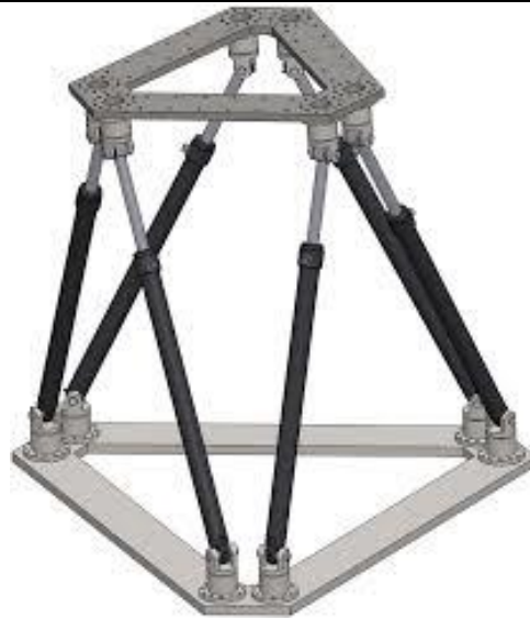
Figure 3: Solid model of the modern 6-6 Stewart platform having prismatic actuators. Source: Stewart-Gough Platform ( Christensen, 2014 )
