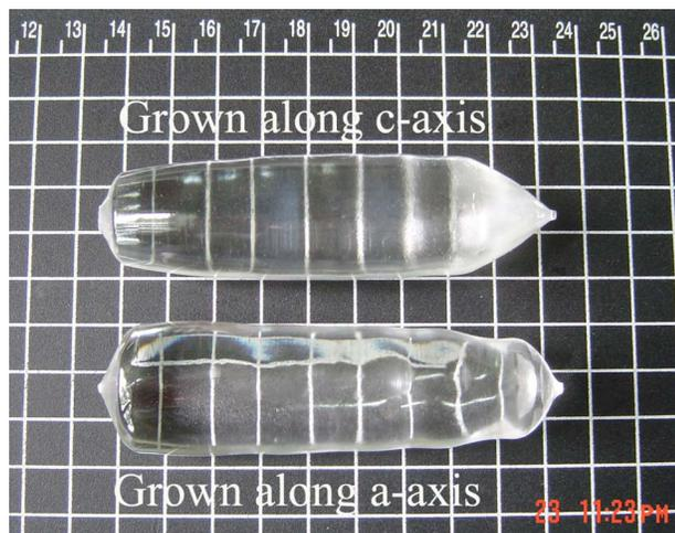
FIG. 1. The photograph of as-grown BaWO<sub>4</sub> crystal.
