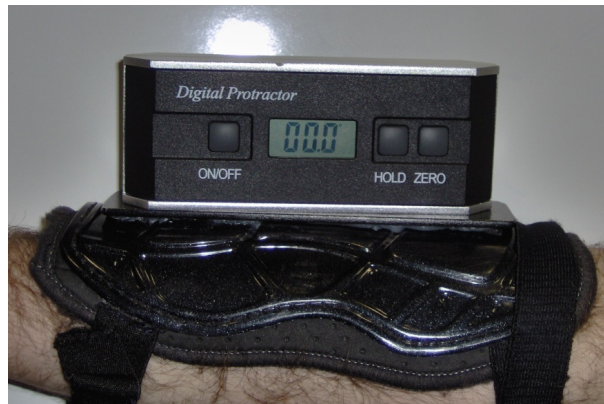
Figure 1. Modified digital inclinometer
