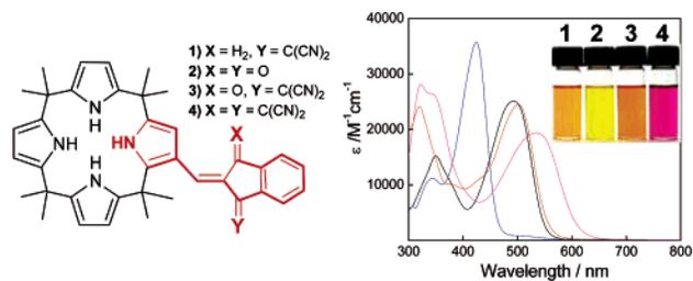
**Figure 4.** Structure and absorption spectra of sensors **1** (black line), **2** (blue line), **3** (orange line), and **4** (pink line) in  $\text{CH}_2\text{Cl}_2$  ( $50 \mu\text{M}$ ). Inset shows solutions.
