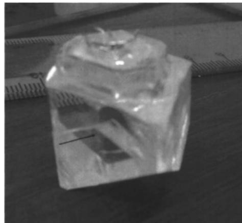
FIG. 3. As-grown KLuW crystal containing fractures with seed orientation along the  $c$  direction.
