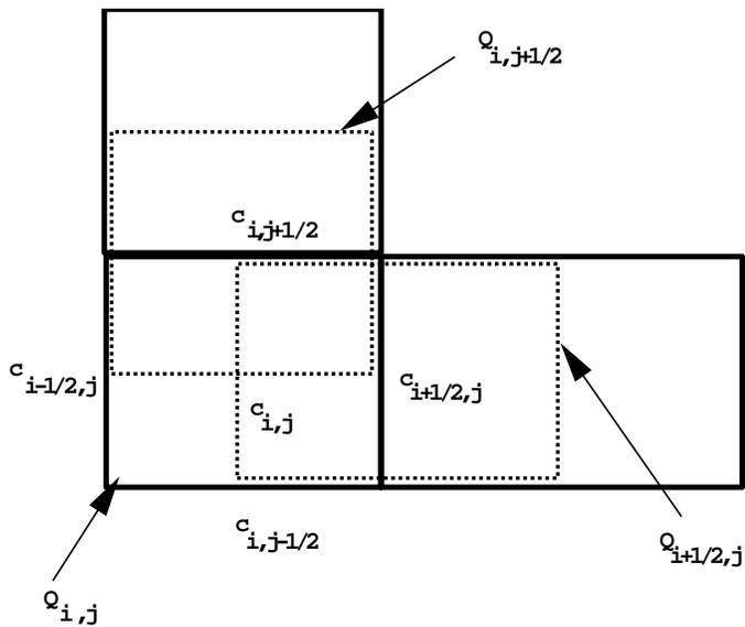
FIG. 2. Dual domain with overlapping covolumes. The dashed boxes  $Q_{i+1/2}$  and  $Q_{i,j+1/2}$  are covolumes;  $c_{i+1/2,j}$  and  $c_{i,j+1/2}$  are the midpoints of the edges of the primal volume  $Q_{i,j}$  whose center is  $c_{i,j}$ .
