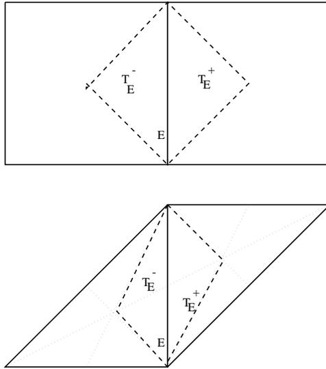
FIG. 1. Primal and dual domains; the dual element (covolume)  $Q'_E = T_E^+ \cup E \cup T_E^-$ .
